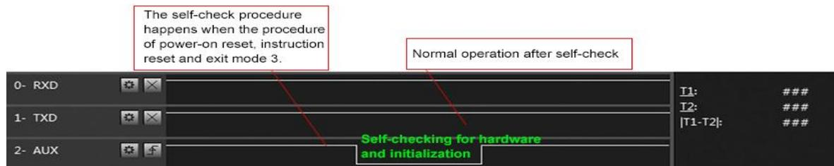
Timing Sequence Diagram of AUX when self-check
