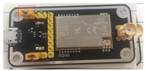
As shown above, connect to jumpers (5V power supply, mode 2), see function details from E32 UART module manual.
