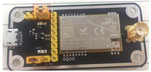
As shown above, connect to jumpers (5V power supply, mode 1), see function details from E32 UART module manual.
