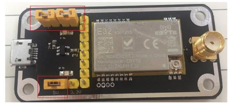
As shown above, connect to jumpers (5V power supply, mode 0), both E32-400TBL-01 are configured this way, open serial port, for data TX and RX, and AUX indicator is blinking.
