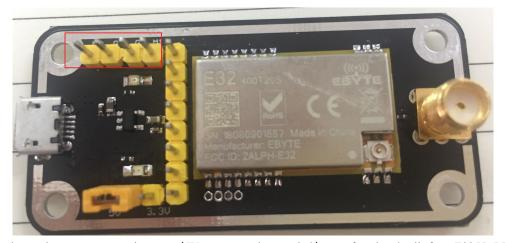
As shown above, connect to jumpers (5V power supply, mode 3), see function details from E32 UART module manual.
