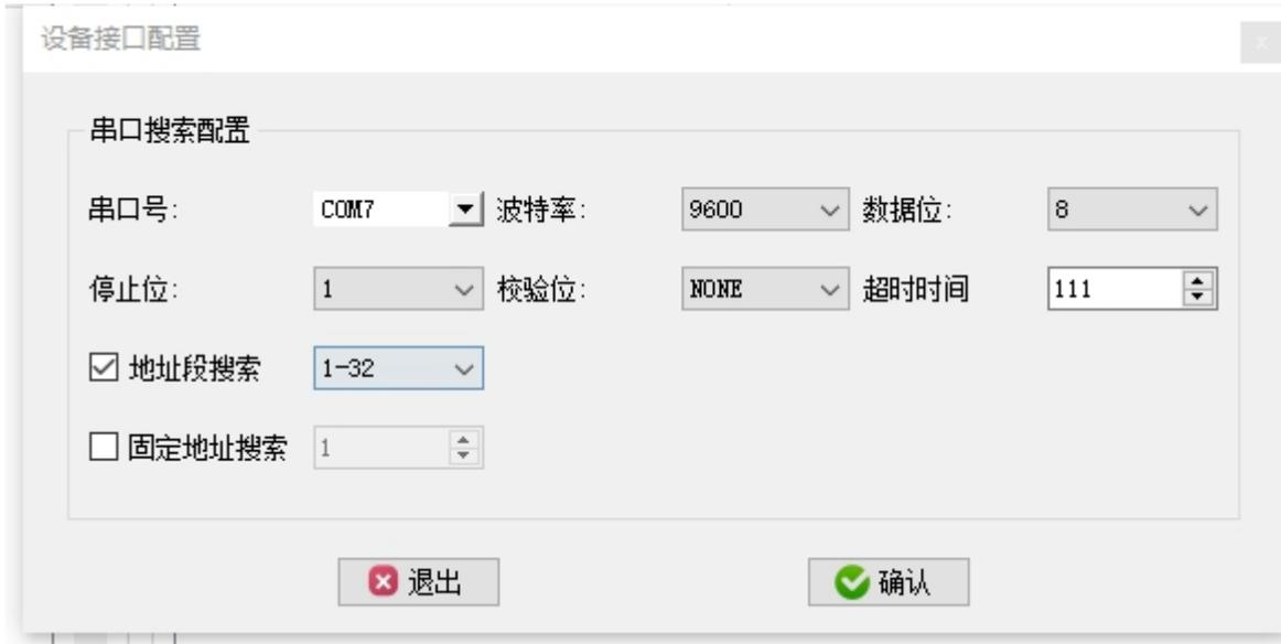
Figure 6-2-3 Serial Port Parameters Window Interface
