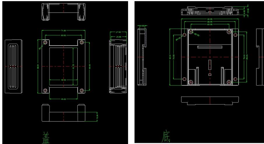
Figure 3-4-2 MA01-AXCX2020-V2/MA01-AXCX2020-V2P/MA01-AXCX3030-V2/MA01-AXCX3030-V2P Dimensional Drawing
