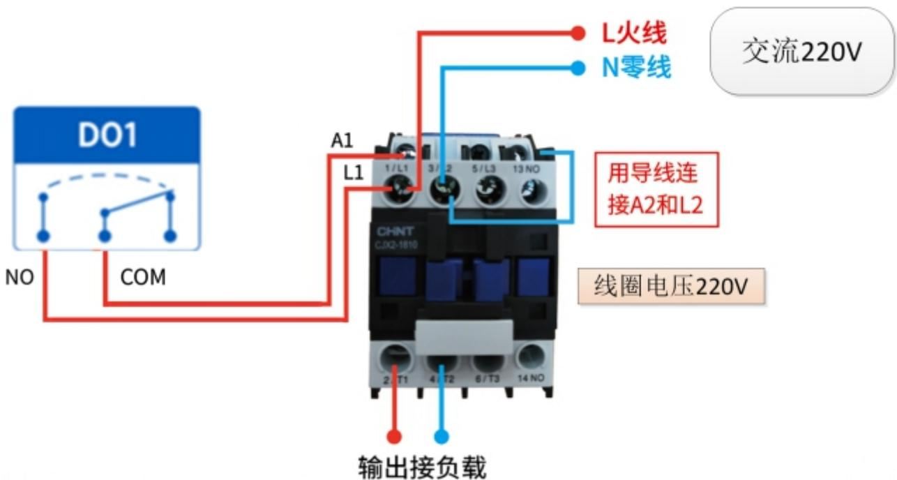
Figure 5-2-2 Wiring Diagram of Output End Control Contactor
